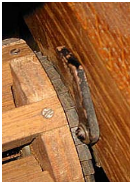
System of blocking of the front roller. Sight of the bobbin and the fixed cog on the side of the roller
