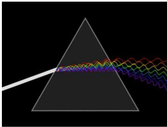
This animation provides a simplified, conceptual view of how various wavelengths that make up white light bend differently as they pass through a prism, resulting in the formation of a rainbow.
