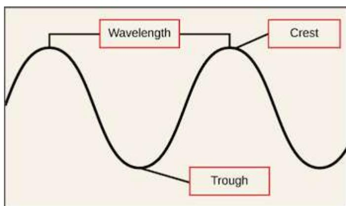
Image of a wave, showing the crests, trough, and wavelength (crest-to-crest distance).
