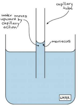
Illustration of water ascending a small tube via capillary action. The thin tube is inserted into a cup of water, and the water climbs up in the tube, reaching a higher level than it does in the cup. Also, the water extends the highest close to the sides of the tube, and dips down in the middle of the tube. This is because the water molecules are more strongly attracted to the sides of the tube than to each other. The curved surface of the water in the capillary tube is called the meniscus.
