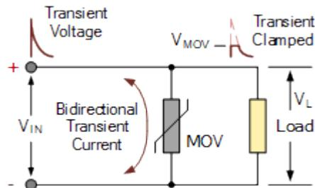
Being a voltage clamping device, metal oxide varistors offer very high resistances when the voltage across its terminals is below its pre-determined breakdown value acting more like a voltage dependent resistor (VDR). When exposed to high transient voltage of either polarity, the electrical characteristics of the device changes and its resistance becomes very small clamping the voltage to a safe level.
