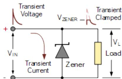
When connected across a supply or across the components being protected, the zener diode is effectively “invisible” until a transient voltage appears as it has a high impedance below its reverse breakdown voltage and a low impedance above its reverse breakdown voltage.
