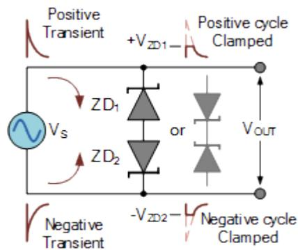
By connecting two zener diodes back-to-back we can now protect both the positive half cycle from overvoltage transients with one zener diode and the negative half cycle with the other.
