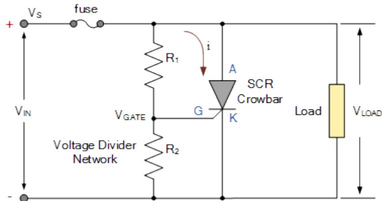
Here a thyristor or SCR is placed across the supply and the load with the voltage divider circuit set up by resistors  $R_1$  and  $R_2$  set to bias the thyristors gate at a level low enough for it not to be triggered “ON” during normal operation. Then the SCR is cut-off and non-conducting.
