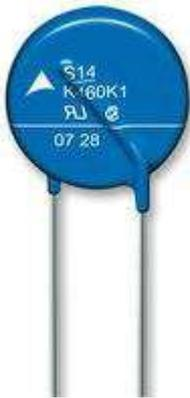
A voltage-clamping device such as an MOV, has a variable impedance depending on the current flowing through the device or on the voltage across its terminal. Under normal steady-state operating conditions, the device offers a high impedance and has therefore no effect on the connected circuit.
