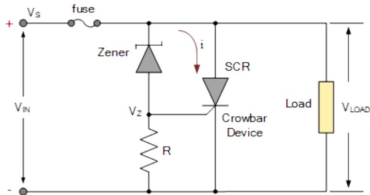
The DC supply voltage,  $V_s$  is monitored by the zener diode which is acting like a transient detection component, and whose zener voltage,  $V_z$  rating determines the voltage level at which the SCR turns on. When the DC supply voltage is lower than the reverse bias rating of the zener diode, the zener diode does not conduct so no voltage or current is applied to the gate of the SCR so remains turned “off”, non-conducting.
