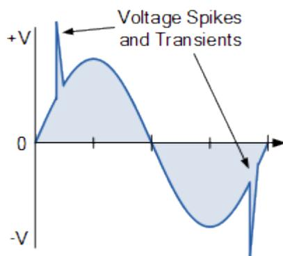
This high  $dv/dt$  transient switching spike can exist either for a very short period of time (milli-seconds or micro-seconds), or they can occur every so often over short periods of time, for example randomly two or three times a day. We must also realise that transients do not always start at zero volts but can be superimposed onto another voltage level. Either way, transients are bad as they can damage electronic equipment and therefore need to be suppressed and controlled.
