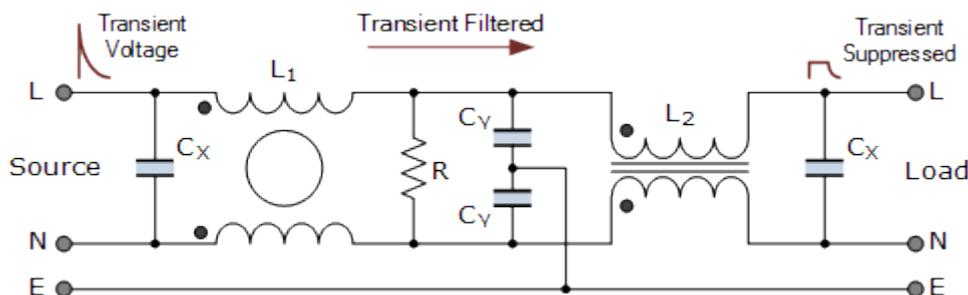
This basic two-stage low-pass AC filter provides a high insertion loss between line-to-line and line-to-ground throughout the frequency range offering effective transient voltage protection by stopping any high-frequency transient and noise from reaching the connected load equipment. Also as well as reducing voltage spikes and transients, these mains power filters can help eliminate any radio-frequency interference or emissions given off by the power supply.
