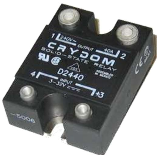
Thus the main advantages solid state relays have over conventional electro-mechanical relays is that they have no moving parts to wear out, and therefore no contact bounce issues, are able to switch both “ON” and “OFF” much faster than a mechanical relays armature can move, as well as zero voltage turn-on and zero current turn-off eliminating electrical noise and transients.
