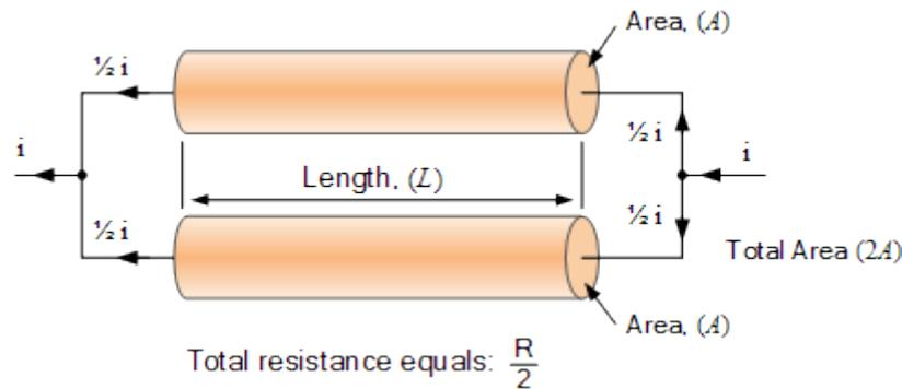
Here by connecting the two conductors together in a parallel combination, we have effectively doubled the total area giving  $2A$ , while the conductors length,  $L$  remains the same as the original single conductor. But as well as doubling the area, by connecting the two conductors together in parallel we have effectively halved the total resistance of the conductor, giving  $1/2R$  as now each half of the current flows through each conductor branch.
