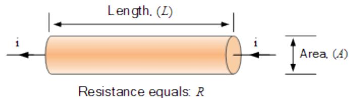
The electrical resistance,  $R$  of this simple conductor is a function of its length,  $L$  and the conductors area,  $A$ . Ohms law tells us that for a given resistance  $R$ , the current flowing through the conductor is proportional to the applied voltage as  $I = V/R$ . Now suppose we connect two identical conductors together in a series combination as shown.
