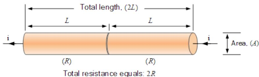
Here by connecting the two conductors together in a series, we have effectively doubled the total length of the conductor,  $2L$  while the cross-sectional area,  $A$  remains exactly the same. But as well as doubling the length, we have also doubled the total resistance of the conductor,
