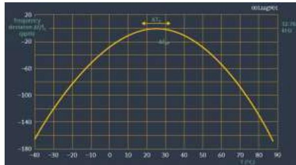
Figure 3: The deviation of frequency with temperature of a typical 32.768kHz crystal.
