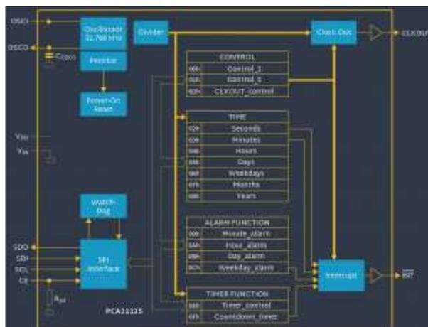
Figure 1: The Internal Circuit Blocks of a PCA21125
