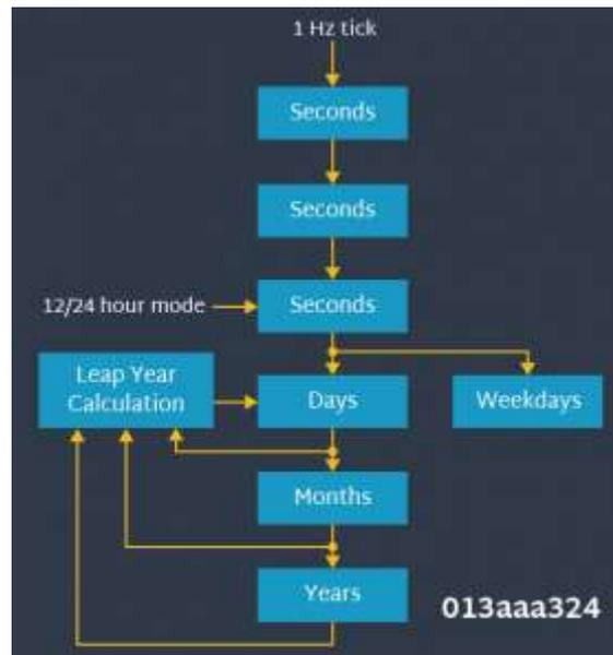
Figure 2: Data flow diagram of a time function.
