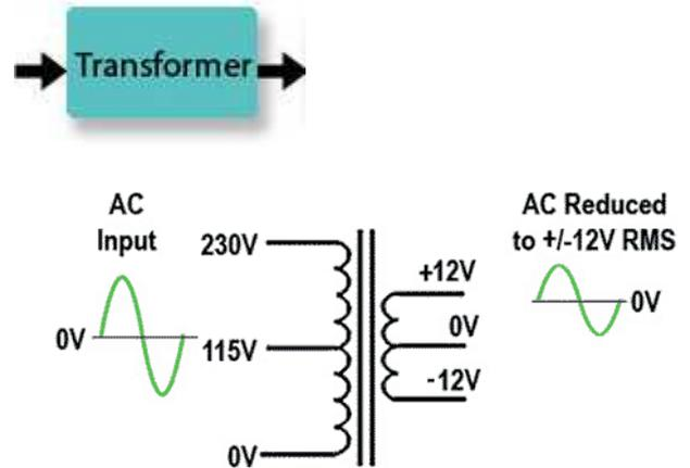
**Fig. 1.1.1 Typical Input Transformer**
