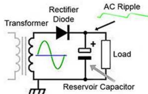
Fig. 1.2.1 The Reservoir Capacitor
