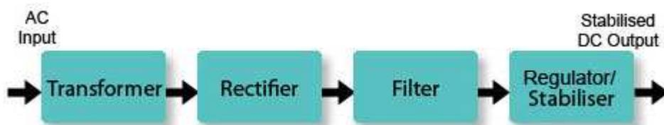
**Fig. 1.0.1 Power Supply Block Diagram**
