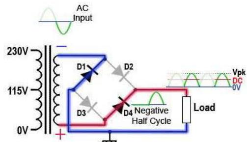
Fig. 1.1.6 Current Flow on the Negative Half Cycle
