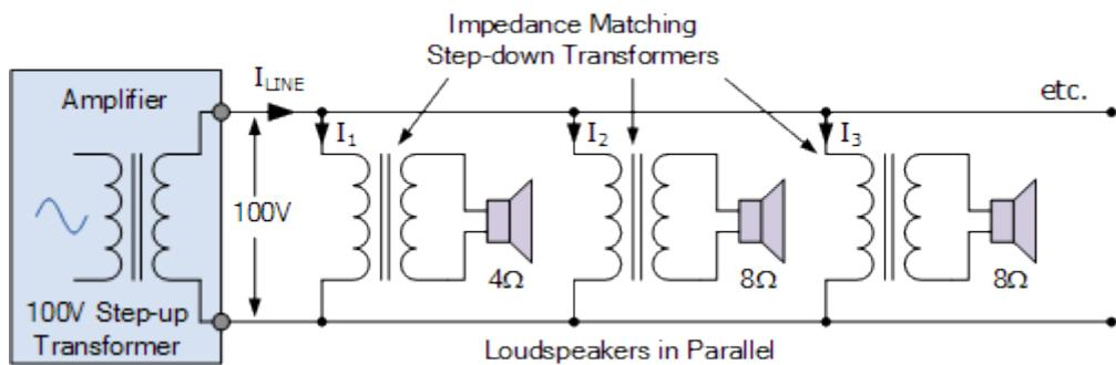
Here the amplifier uses a step-up transformer to provide a constant 100 volts transmission line voltage at reduced current, for a given power output. The loudspeakers are connected together in parallel with each speaker having its own impedance matching step down transformer to reduce the secondary voltage and increase the current, thereby matching the 100V line to the low impedances of the loudspeakers.
