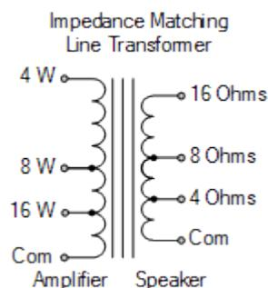
Generally transmission line matching transformers have multiple connections called tapping points on the primary winding allowing for suitable power levels (and therefore sound volume) to be selected for each individual loudspeaker. Also, the secondary winding has similar tapping points offering different impedances to match that of the connected loudspeakers.
