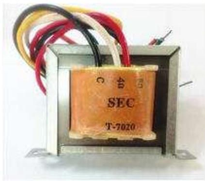
When an AC signal is applied to the primary input winding, a corresponding AC signal appears on the output secondary winding due to the inductive coupling of the soft iron core. The turns ratio between the input and output wire coils provides either an increase or a decrease of the applied signal as it passes through the transformer.
