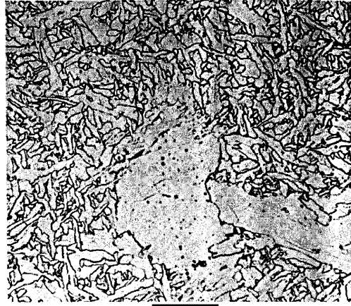
Figure W21.21. Coarse acicular ferrite, a disorganized structure of randomly oriented ferritic plates, is shown in a weld zone along with polygonal ferrite. The horizontal bar corresponds to 20 \mu\text{m} . (From ASM Handbook, 9th ed., Vol. 9, Metallography and Microstructures , ASM International, Materials Park, Ohio, 1985, p. 585.)
