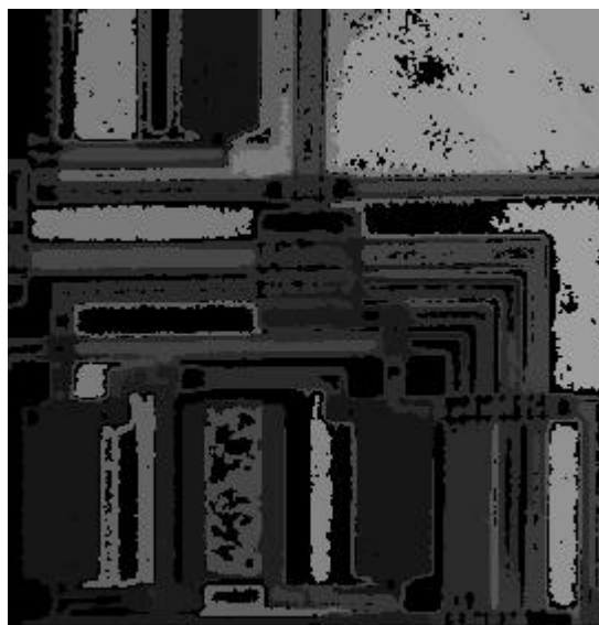
Figure 2: The result of region growing procedure on CIRCUIT using a threshold of 20 and randomly selected seeds.
