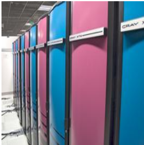
Louhi: Cray XT4/XT5 with 2.3 GHz 4-core AMD Opteron. All-in-all 9424 cores and Peak power of 86.7 Tflops.
