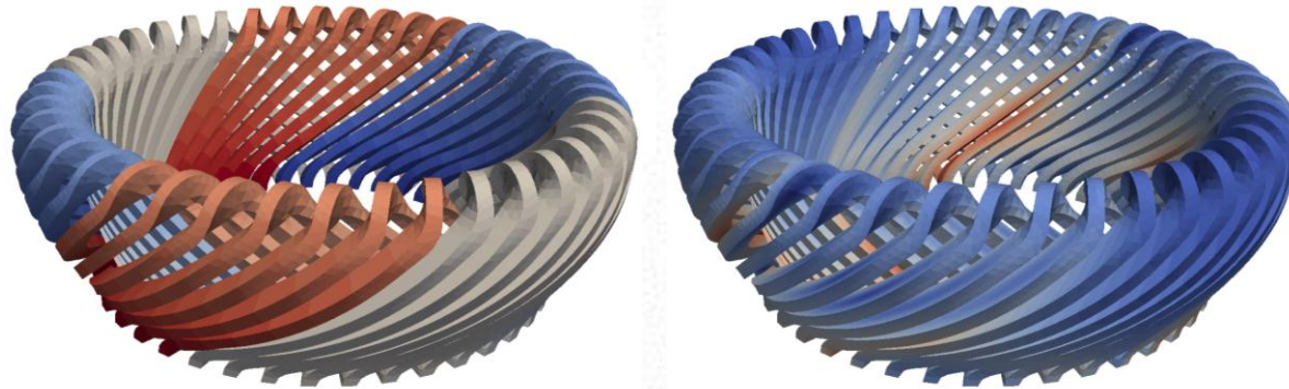
Magnetic field strength (left) and electric potential (right) of an electrical engine end-windings. Meshing M. Lyly, ABB. Simulation J. Ruokolainen, CSC, 2013.
