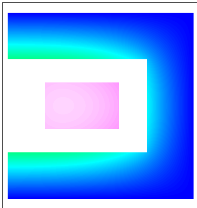
Figure 1.1: Temperature distribution in the radiation heat transfer problem
