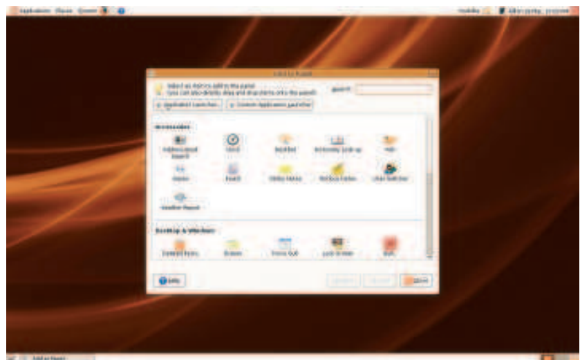
» Right-click on a spare part of a panel, then choose Add To Panel – there are lots of things you can try here, but don't go overboard!
