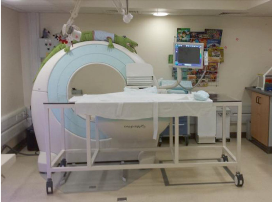
Fig. 9.2 Custom made cut out gamma camera acquisition table
