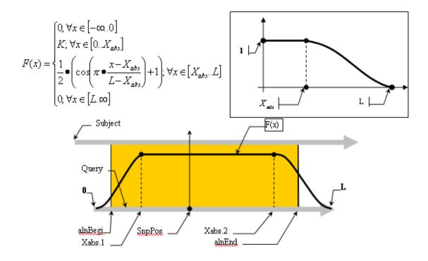
Alignment Quality, "Q", can be calculated using the following equation:
