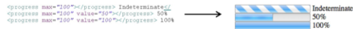
Figure 6 – Progress indicators available through this HTML5 feature and the code for each
