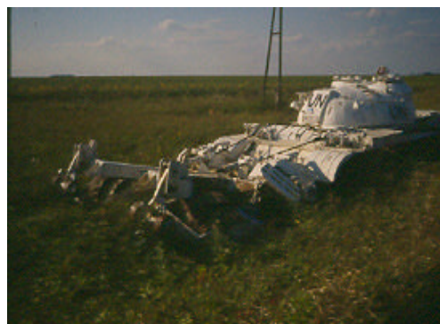
Figure 38. This machine is mounted on a tank body and uses a roller and plough in combination. It suffers from many of the disadvantages of both tools (photo by the author, 1996).
