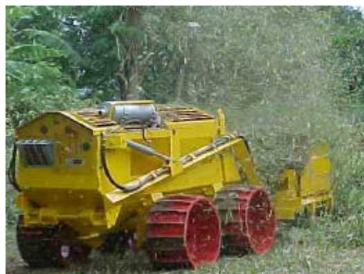
Figure 33. The TEMPEST vegetation-cutting machine working in Cambodia. The TEMPEST was designed and built by Development Technology Workshop (DTW) (photograph by DTW).
