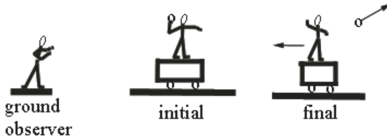
Figure 11.6 Recoil of a person on cart due to thrown ball
