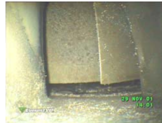
Corrosion Inside TF-34 Engine (S-3)
