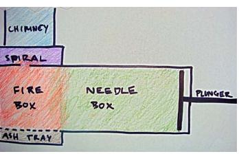
chamber and simply keeping the firebox and the spiral on top, but using the pine needle as a primary fuel source and a secondary fuel source. The spiral would allow for the latter to occur, by elongating the burn path and creating a horizontal channel. The pine needles needed to be compacted to control the burn, but there was no pre-processing required.
