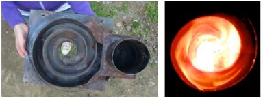
Figure 2a. Top view of the spiral component.Figure 2b. Flames of the secondary burn traveling around the spiral.
