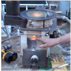
Figure 4. The hand in this photo is pointing at an air inlet. Below that is the ash tray.
