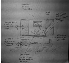
from the shoot and begin burning the supply along the tube. Even with a short chimney, there was not enough controlled airflow, and the gas released by the pine needles, was inefficiently being unused and escaped.
