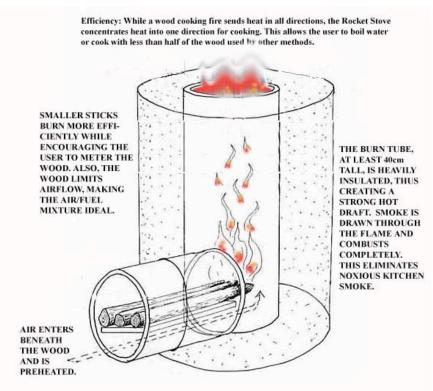
Figure: Diagram of the Rocket Stove Combustion Process-
