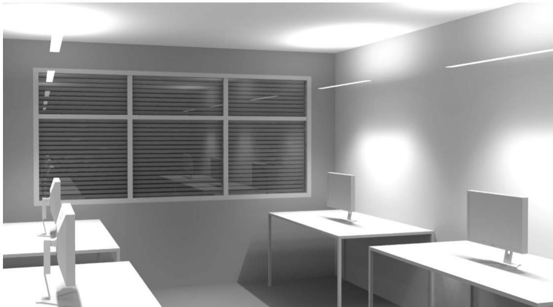
Fig 2: Perspective view of the MIT reference office at MIT equipped with six direct/indirect suspended LED modules
