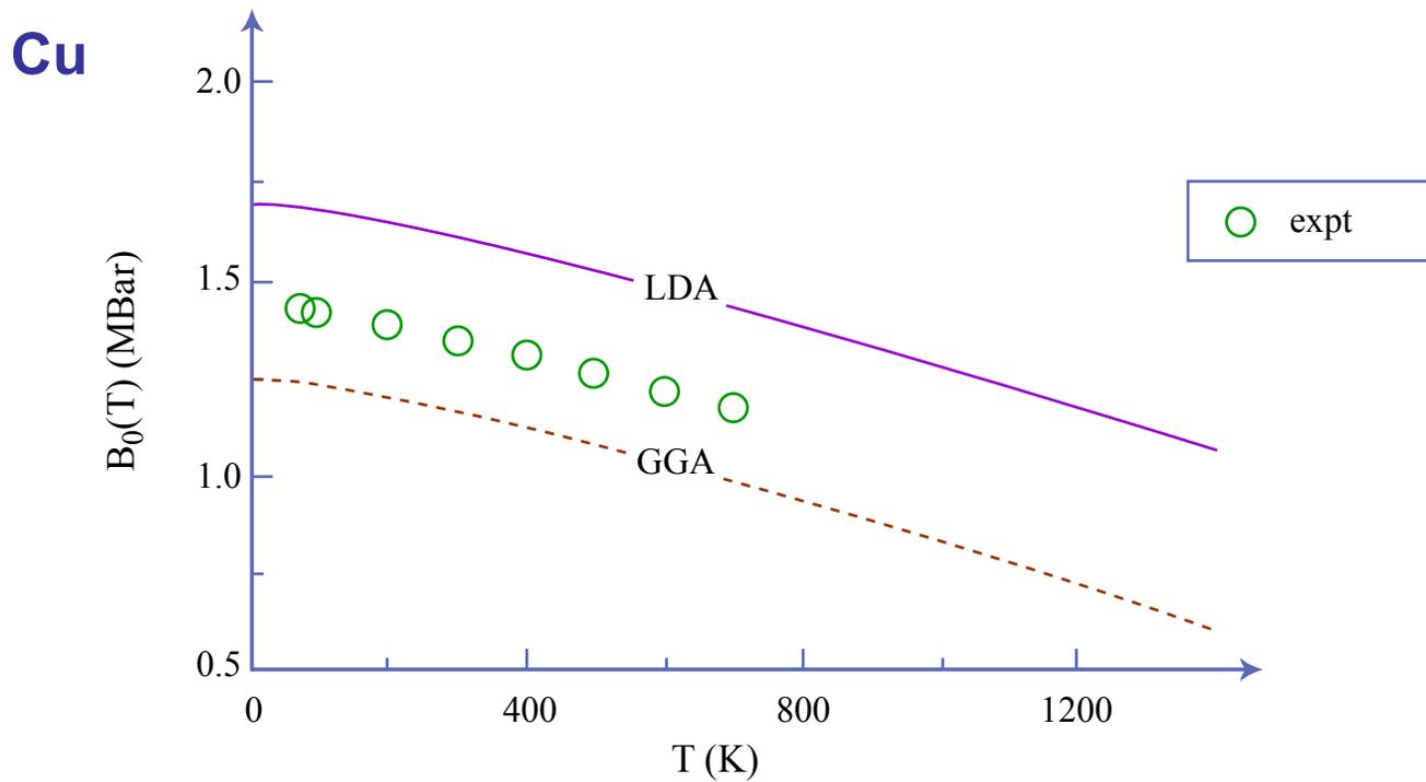
Variation with temperature of the bulk modulus  $B_0$ . At all temperatures, the LDA (solid line) overestimates  $B_0$  and the GGA (dashed line) underestimates it; however,  $\partial B_0 / \partial T$  is approximately the same for the LDA, GGA, and experimental values.
