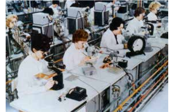
Microelectronic production: Manufacturing the Apollo Guidance Computer, ca. 1966. Photo: Raytheon, from the files of Jack Poundstone.
