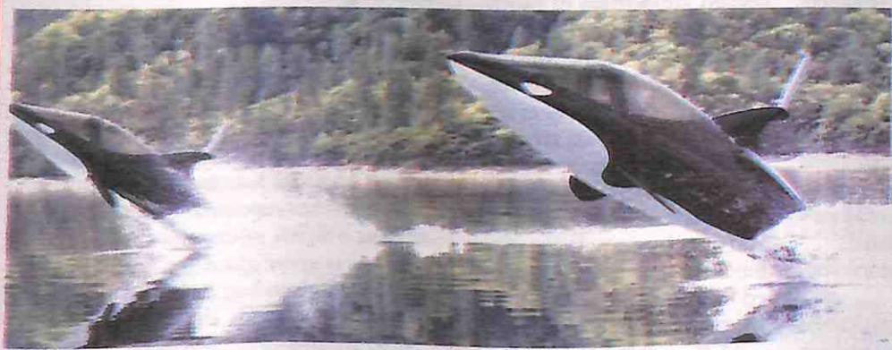
WAVE BRAKER: The Seabreacher operates more like an aircraft with full three axis of control - pitch, roll, and yaw.
