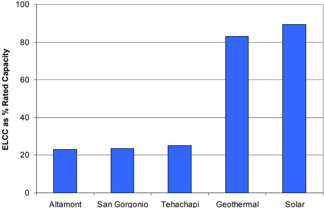
Figure 6 shows other capacity credit values for wind measured by ELCC. Many of the results came from the MN/DOC study recently completed by Enernex. The ELCC values from that study ranged from the upper 20s to low-mid 30s, depending on the modeling technique used for the scenario and whether wind is the currently installed wind or prospective wind expected to be developed within the study horizon.
