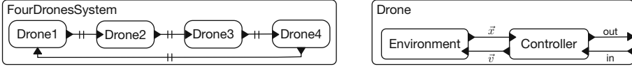
Fig. 2. The AADL architecture of four drones (left), and a drone component (right).
