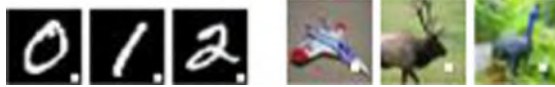
Fig. 3. Example poisoned data for MNIST (left) and CIFAR-10 (right). The backdoor is embedded as the white square at the bottom right corner of each image. When the backdoor appears, the poisoned MNIST model will classify the input as “7” and the poisoned CIFAR-10 model will classify it as “horse”.
