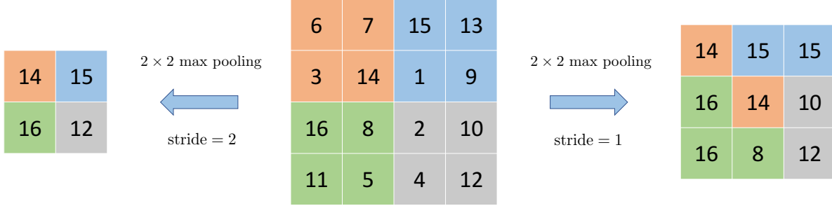
Figure 6: A 2 \times 2 max pooling layer extracts the maximum of 2 by 2 neighboring pixels / features across the spatial dimension.
