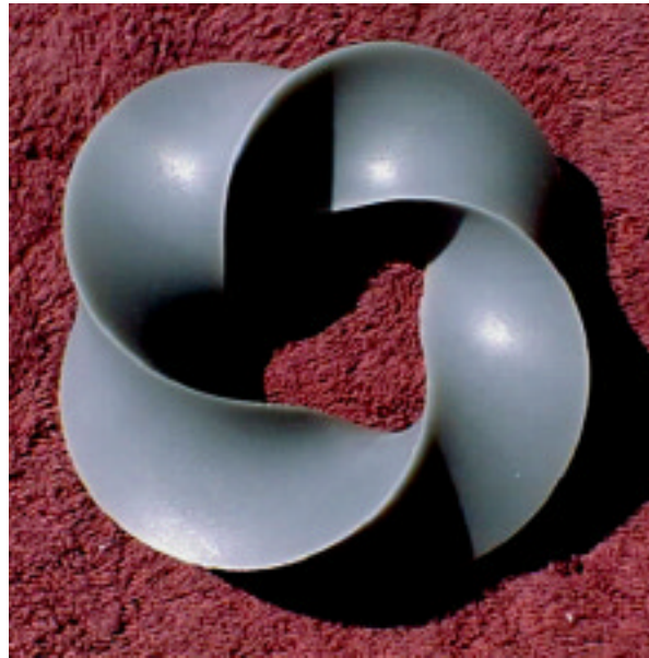
Figure 16.5c: the torus created by the 3D Systems ThermaJet system
