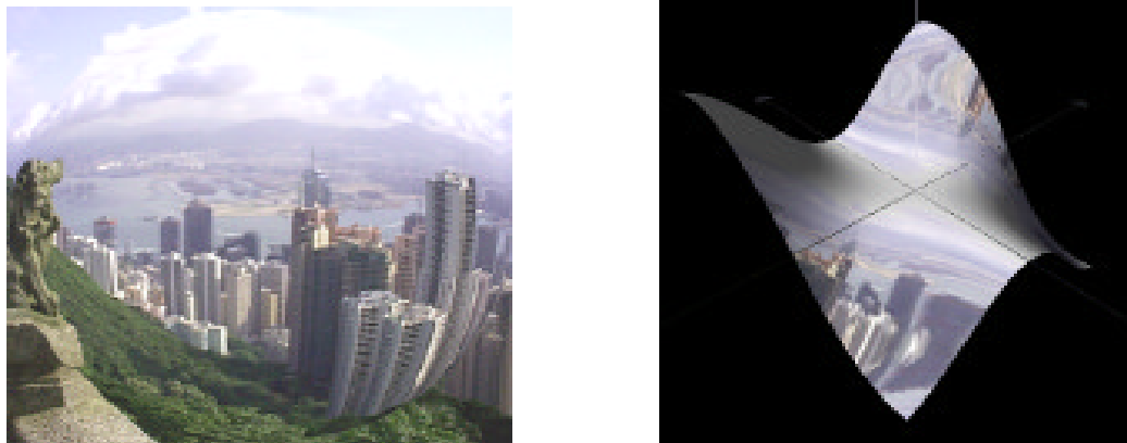
Figure 11.6: the original texture for an environment map (left) and the map on a surface (right)
