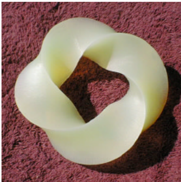
Figure 16.5d: the torus created by the 3D Systems stereolithography system
