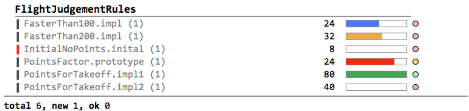
Figure 11.1 An assessment that shows an overview of the efforts spent for work packages associated with requirements. The number is the estimated effort for the work package. The progress bar shows the degree of completion, and the color highlights the effort spent relative to the estimated effort: green = finished with estimated or less effort, blue = in progress, percentage of effort spent is less than percentage finished, yellow = in progress, percentage of effort spent is more than percentage finished, red = effort spent more than estimated. Note how the projectional editor is used to render graphical progress bars in the editor of an assessment.
