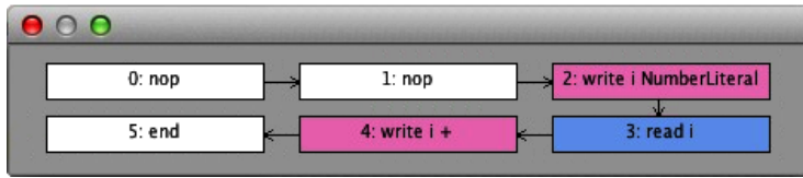
Figure 9.9 An example of a dataflow for a simple C function. The dataflow graph for a program element can be shown by selecting Language Debug -> Show dataflow Graph from the element's context menu. This will render the dataflow graph graphically and constitutes a good debugging tool when building custom dataflow graphs and analyses.
