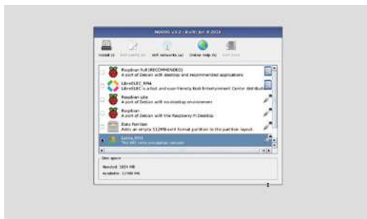
▲ NOOBS (New Out Of Box Software) is used to install operating systems such as Lakka on Raspberry Pi
