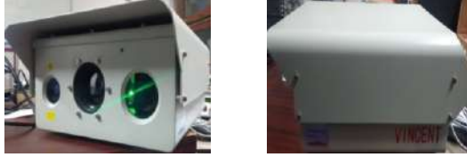
Figure 2. The “VINCENT HD and Night vision IR camera” used for the thermal imaging
