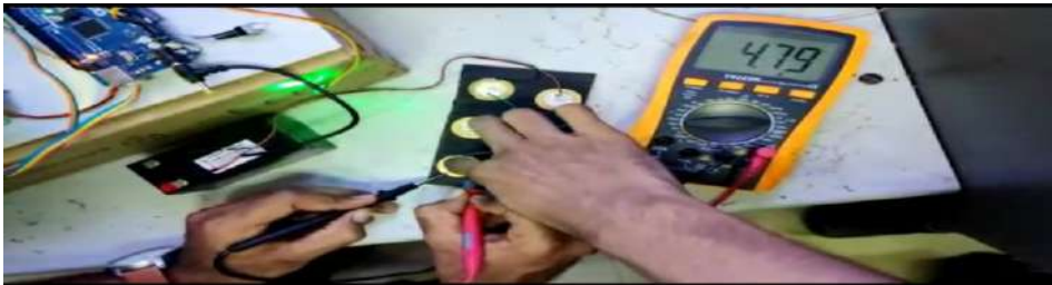
Figure 2. measurement of voltage generated at piezoelectric setup using multimeter.
