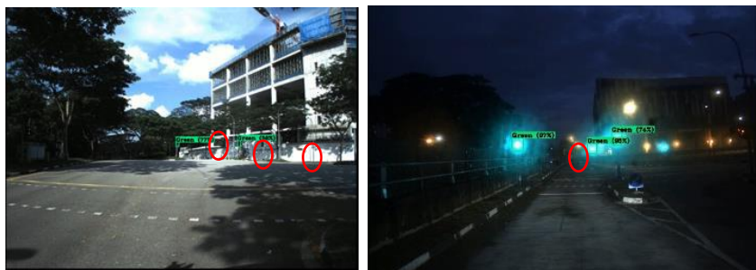
Figure 5. Inconsistent Traffic Light Recognition
