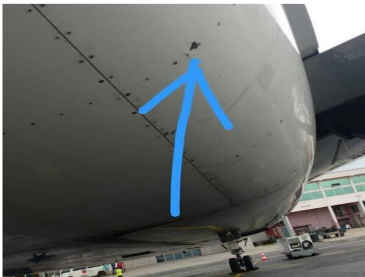
Figure 6. Example of a rare defect: Gunshot Damage of an A330-300 hit by a bullet in Congo on April 11 th , 2020.
