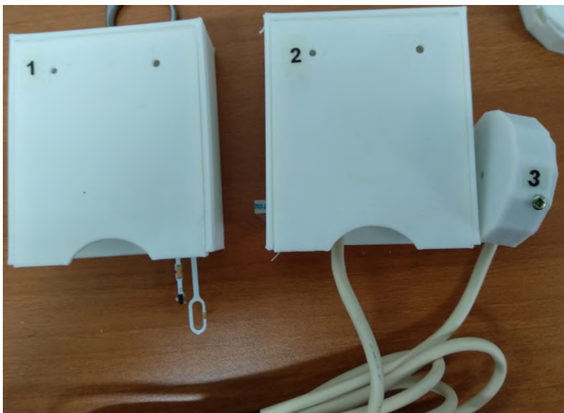
Figure 4. Modules of electronic instrument. 1 is the outdoor variable measurement module. 2 is the indoor variable measurement module and 3 is the warning signal for the final user.
