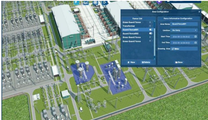
Figure 3. Illustration of the virtual working area setting based on three-dimensional electric fence.
