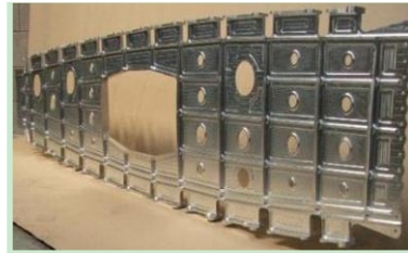
Figure 2. A wing rib of Airbus plane (15V2).
