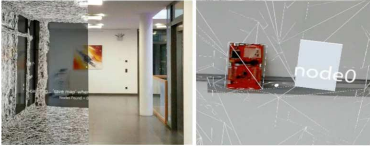
Figure 4. Visualization of a 3D scanned mesh for remote view (left) and augmented node information during deployment (right).
