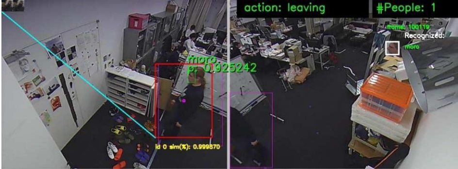
Figure 10. An example of described scene. The action and # people in the scene is shown on the top. On the right the recognized human from the sequence. In the region of interest tracked (red), the current associated label (green) with relative likelihood, and similarity (yellow).
