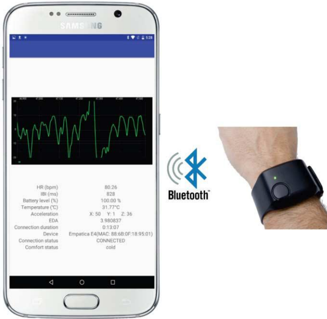
Figure 1. Real-time thermal comfort prediction system —An Empatica E4 wristband is used to record a photoplethysmogram (PPG) signal. An inter-beat interval (IBI) signal is extracted from the PPG, sent to a smartphone, and used to calculate pulse rate variability indices (PRV). These indices are thereafter used to predict, in real-time, the comfort state of the wearer of the E4 device
