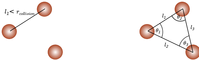
Figure 1. Visualization of bonding at runtime. Left: If two particles are closer than the collision distance, the algorithm aims to find a third particle within the collision distance to establish a triangular bonding structure. Right: The bonding structure consists of three angular bonds (indicated as \theta_1, \theta_2, \theta_3 ) as well as three distance-based bonds (indicated as l_1, l_2, l_3 ) between the particle pairs. If no third particle could be found, only the distance bond l_1 is created.
