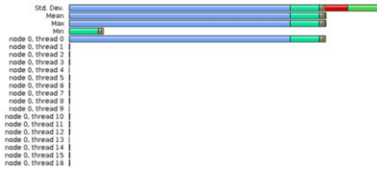
Figure 4. TAU profile results for move_grid 's execution time per call. Most of the time was spent by the main thread.
