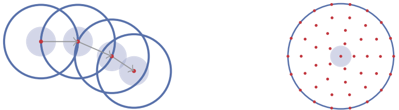
a) Illustration of footsteps of agent i . The circles (blue) indicate the actual step radius \lambda_i and the shaded area (blue) represents the agent torso of radius r_p . b) Approximation of P_i by equidistant points inside the step circle.
