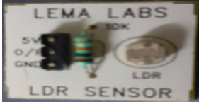
Figure 5. LDR sensor light detector
