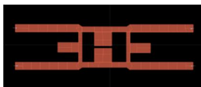
Figure 6. Layout of compact Branchline coupler using ADS software
