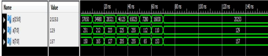
Figure 5. Simulation result of the Multiplier
