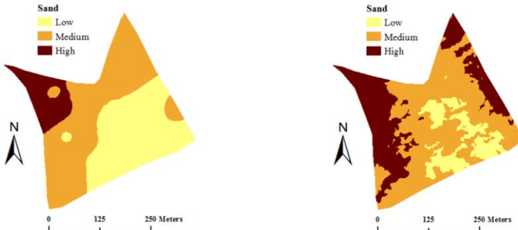
Figure 5. Comparison between (a) the 18 laboratory reference point and (b) the full-point on-line visible and near infrared (Vis-NIR) predicted maps for sand content.
