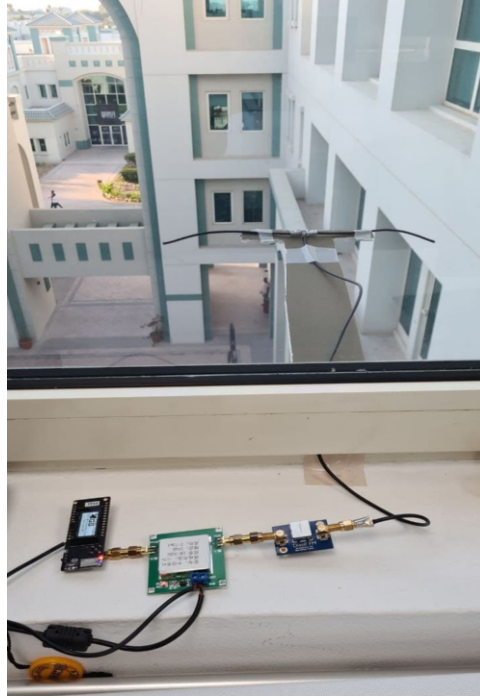
Figure 7. Ground Station setup at the Robotics Lab, Middlesex University, Dubai.
