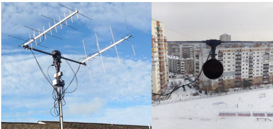
Figure 6. Yagi UDA antenna and simple dipole antenna
