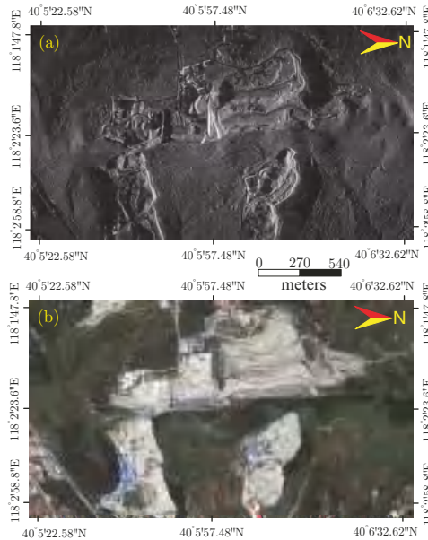
Figure 12. Monostatic spotlight image processed using MoBulk_FFBP. (a) The monostatic spotlight image; (b) the optical image of the imaging area from Google Earth.
