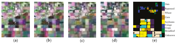
Figure 4. Study area. (a–d) RGB composite images of the filtered multi-temporal UAVSAR data (17 June, 22 June, 5 July, and 17 July in 2012 respectively) with Pauli basis; (e) Ground-truth map for seven known land covers.
