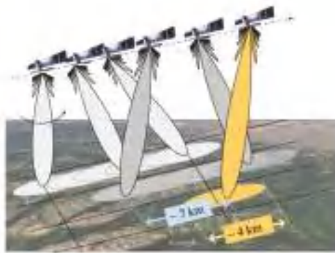
Figure 1. Sketch of TOPSAR acquisition mode, here represented as the three swaths Sentinel-1 IW.
