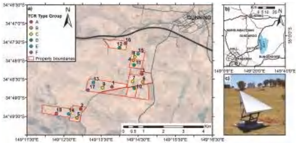
Figure 6. (a) Map showing the 18 TCR deployment sites at the Gunning test site coloured by type group (Table 2). The background image is a Landsat-8 RGB-composite optical image acquired on 15 January 2014 with 30 m pixel resolution. Red polygons outline the boundaries of the property available for the experiment. (b) Overview map showing the location of the Gunning test site (red polygons) in relation to Canberra, Australia; (c) photo of TCR number 7 as deployed at the Gunning test site.
