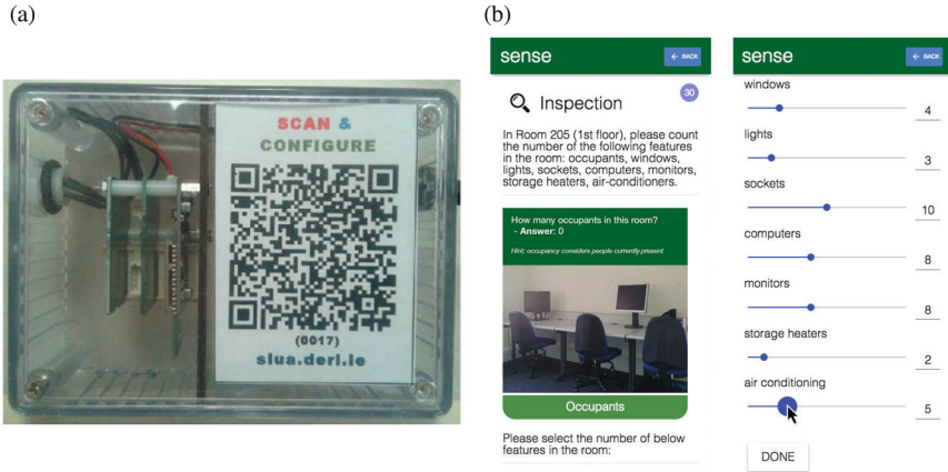
Fig. 9.3 Examples of a human task to enrich entities. (a) Sensor metadata enrichment. (b) Entity enrichment (e.g. room features) [4]
