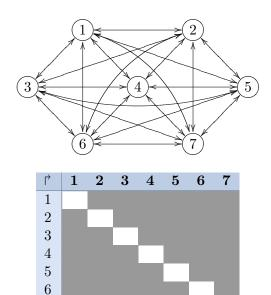
**Figure 3.8:** A completely linked network with symmetric connections and without direct recurrences. In the Hinton diagram only the diagonal is left blank.
