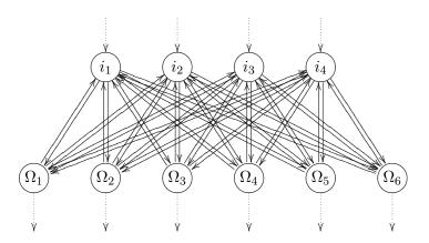
Figure 11.1: Simplified illustration of the ART network structure. Top: the input layer, bottom: the recognition layer. In this illustration the lateral inhibition of the recognition layer and the control neurons are omitted.
