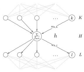
**Figure 5.11:** Illustration of the position of our neuron h within the neural network. It is lying in layer H, the preceding layer is K, the subsequent layer is L.
