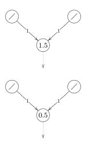
**Figure 5.4:** Two singlelayer perceptrons for Boolean functions. The upper singlelayer perceptron realizes an AND, the lower one realizes an OR. The activation function of the information processing neuron is the binary threshold function. Where available, the threshold values are written into the neurons.
