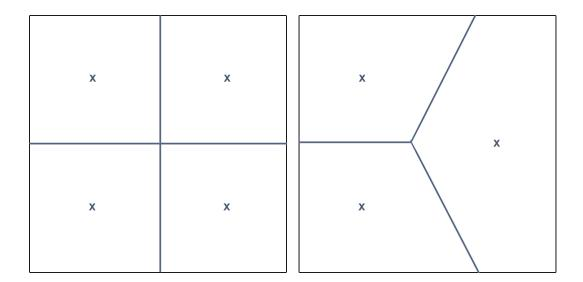
Figure 9.1: BExamples for quantization of a two-dimensional input space. DThe lines represent the class limit, the imes mark the codebook vectors.
