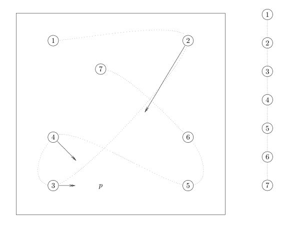
**Figure 10.4:** Illustration of the two-dimensional input space (left) and the one-dimensional topolgy space (right) of a self-organizing map. Neuron 3 is the winner neuron since it is closest to p. In the topology, the neurons 2 and 4 are the neighbors of 3. The arrows mark the movement of the winner neuron and its neighbors towards the training sample p.
