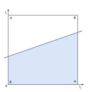
**Figure 5.7:** Linear separation of n=2 inputs of the input neurons  $i_1$  and  $i_2$  by a 1-dimensional We assume a positive weight  $w_{i_2,\Omega}$ , the in-straight line. A and B show the corners belonging to the sets of the XOR function that are to be separated.
