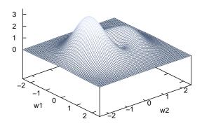
**Figure 5.5:** Exemplary error surface of a neural network with two trainable connections  $w_1$  und  $w_2$ . Generally, neural networks have more than two connections, but this would have made the illustration too complex. And most of the time the error surface is too craggy, which complicates the search for the minimum.
