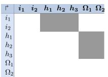
Figure 3.3: A feedforward network with three layers: two input neurons, three hidden neurons and two output neurons. Characteristic for the Hinton diagram of completely linked feedforward networks is the formation of blocks above the diagonal.
