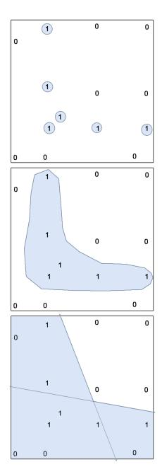
**Figure 4.1:** Visualization of training results of the same training set on networks with a capacity being too high (top), correct (middle) or too low (bottom).
