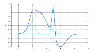
**Figure 6.4:** Four different Gaussian bells in one-dimensional space generated by means of RBF neurons are added by an output neuron of the RBF network. The Gaussian bells have different heights, widths and positions. Their centers  $c_1, c_2, \ldots, c_4$  are located at 0, 1, 3, 4, the widths  $\sigma_1, \sigma_2, \ldots, \sigma_4$  at 0.4, 1, 0.2, 0.8. You can see a two-dimensional example in fig. 6.5 on the following page.
