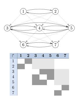
Figure 3.7: A network similar to a feedforward network with laterally recurrent neurons. The direct recurrences are represented by solid lines. Here, recurrences only exist within the layer. In the Hinton diagram, filled squares are concentrated around the diagonal in the height of the feedforward blocks, but the diagonal is left uncovered.
