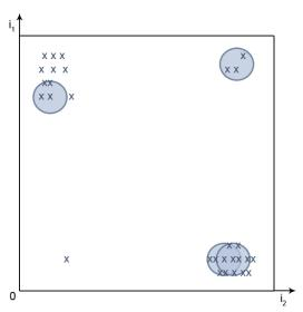
**Figure 6.8:** Example of an uneven coverage of a two-dimensional input space by applying radial basis functions. The widths were fixedly selected, the centers of the neurons were randomly distributed throughout the training patterns. This distribution can certainly lead to slightly unrepresentative results, which can be seen at the single data point down to the left.
