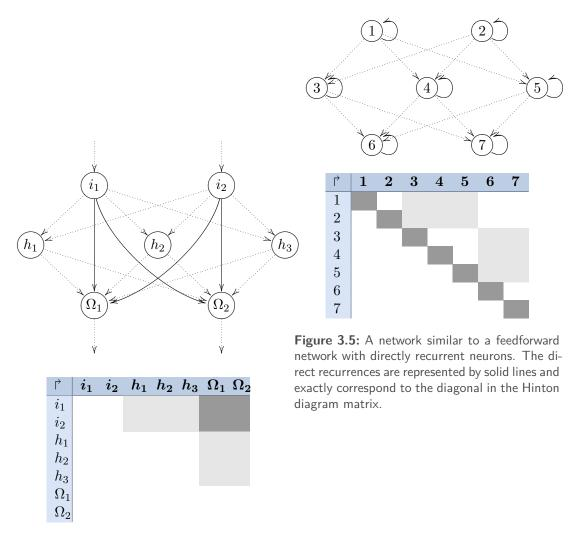
**Figure 3.4:** A feedforward network with short-cut connections, which are represented by solid lines. On the right side of the feedforward blocks new connections have been added to the Hinton diagram.
