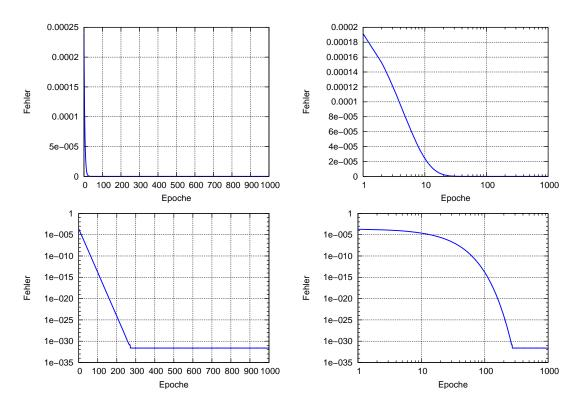
**Figure 4.2:** All four illustrations show the same (idealized, because very smooth) learning curve. Note the alternating logarithmic and linear scalings! Also note the small "inaccurate spikes" visible in the sharp bend of the curve in the first and second diagram from bottom.
