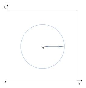
**Figure 6.2:** Let  $c_h$  be the center of an RBF neuron h. Then the activation function  $f_{acth}$  is ra- **6.2.1 Information processing in** dially symmetric around  $c_h$ .
