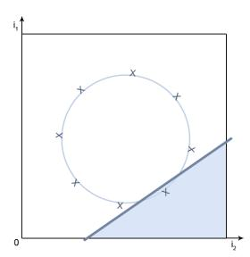
**Figure 5.15:** Illustration of the functionality of 8-2-8 network encoding. The marked points represent the vectors of the inner neuron activation associated to the samples. As you can see, it is possible to find inner activation formations so that each point can be separated from the rest of the points by a straight line. The illustration shows an exemplary separation of one point.
