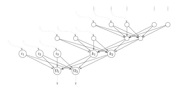
**Figure 7.4:** Illustration of the unfolding in time with a small exemplary recurrent MLP. **Top:** The recurrent MLP. **Bottom:** The unfolded network. For reasons of clarity, I only added names to the lowest part of the unfolded network. Dotted arrows leading into the network mark the inputs. Dotted arrows leading out of the network mark the outputs. Each "network copy" represents a time step of the network with the most recent time step being at the bottom.
