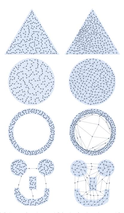
**Figure 10.6:** End states of one-dimensional (left column) and two-dimensional (right column) SOMs on different input spaces. 200 neurons were used for the one-dimensional topology,  $10 \times 10$  neurons for the two-dimensionsal topology and 80.000 input patterns for all maps.
