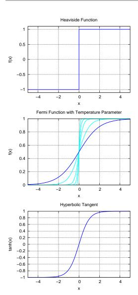
**Figure 3.2:** Various popular activation functions, from top to bottom: Heaviside or binary threshold function, Fermi function, hyperbolic tangent. The Fermi function was expanded by a temperature parameter. The original Fermi function is represented by dark colors, the temperature parameters of the modified Fermi functions are, ordered ascending by steepness,  $\frac{1}{2}$ ,  $\frac{1}{5}$ ,  $\frac{1}{10}$  und  $\frac{1}{25}$ .
