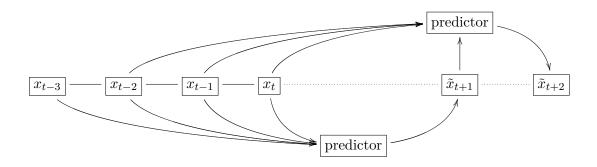
**Figure B.3:** Representation of the two-step-ahead prediction. Attempt to predict the second future value out of a past value series by means of a second predictor and the involvement of an already predicted value.
