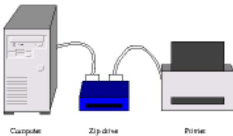
This technique relies on certain “special signals” being invisible to devices that aren’t watching for them. This tends to mean only changing the data signals and leaving the control signals alone. IEEE 1284.3 documents a standard protocol for daisy-chaining devices together with parallel ports.
