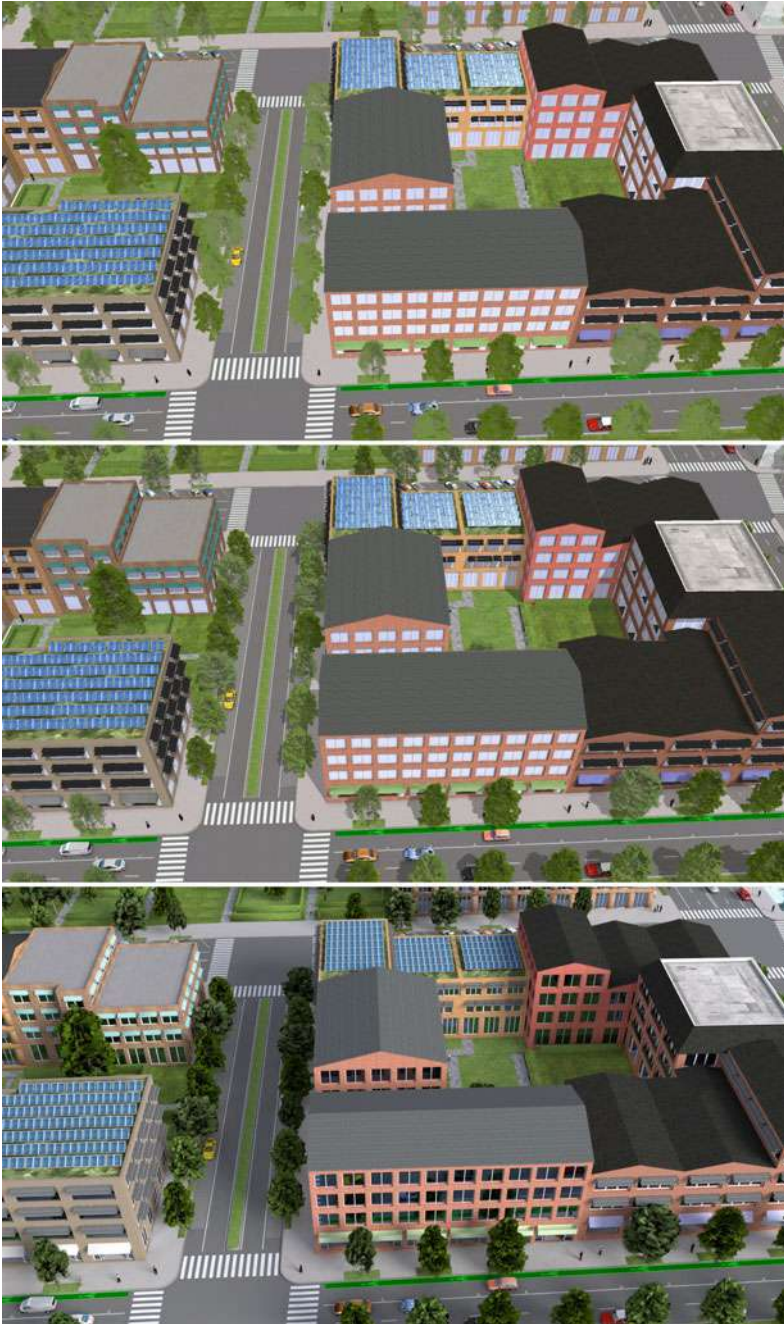
Fig. 35.17 Top: CityEngine’s default OpenGL real-time renderer without ambient occlusion or shadows. Middle: with ambient occlusion and shadows. Bottom: Blender’s Cycles renderer takes 12 min to render this image with soft shadows and reflective glass. The mesh was exported to Blender in the OBJ format
