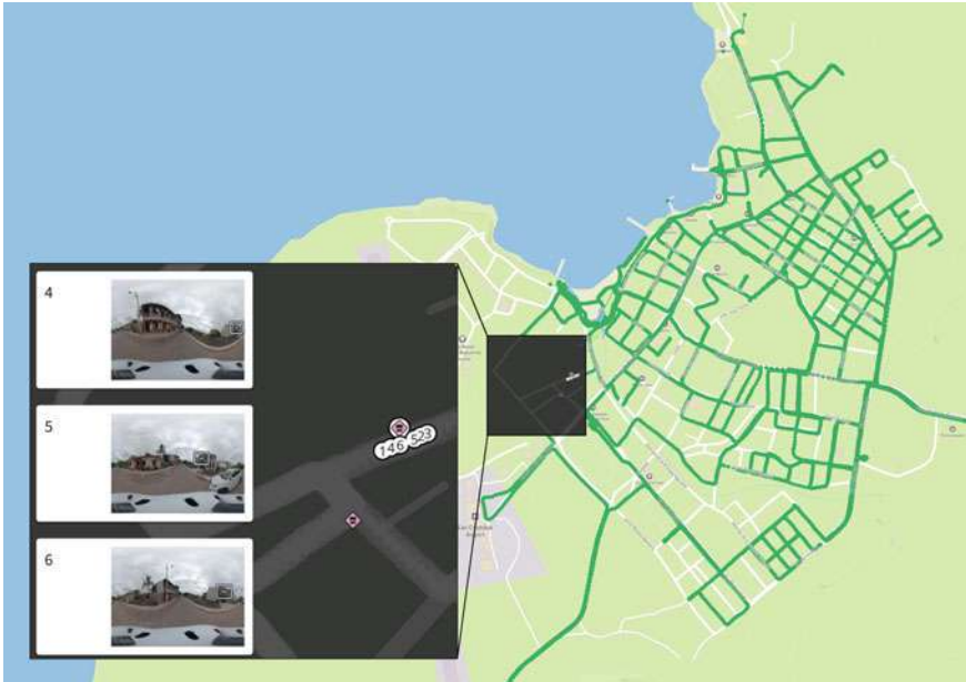
Fig. 4.3 The imagery covers most of the accessible street network of Puerto Baquerizo Moreno on San Cristóbal, Galapagos. The green dots show the locations of all 360-degree imagery produced by us. When a series of images are available along a street, objects can be identified and geolocated. The inset depicts a situation in which the same store sign is recognized in six different images in the right inset panel, taken from slightly different locations, of which three are shown in the left inset panel. Map designs are from Mapillary (2019) and OpenStreetMap (2019)
