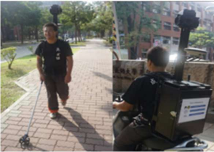
Fig. 25.7 Example of portable mobile mapping systems
