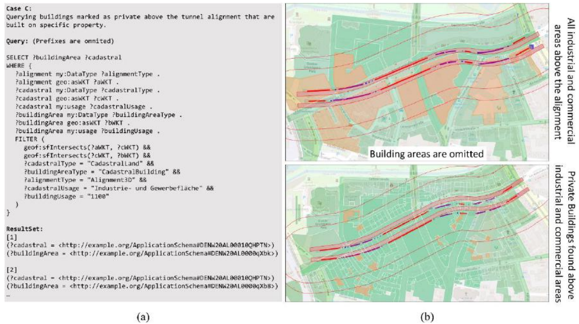
Figure 8: The query performed in Case C (a) and the results visualized in the project environment (b)
