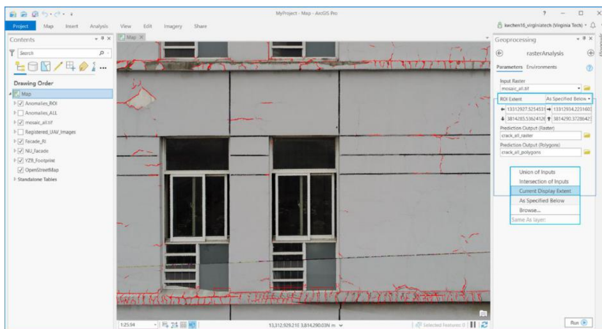
Figure 8: Execution of developed GIS tools for the detection of crack pixels using trained models
