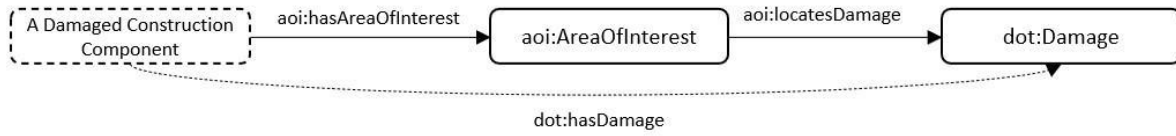
Figure 3: Extension example of AOI for DOT support
