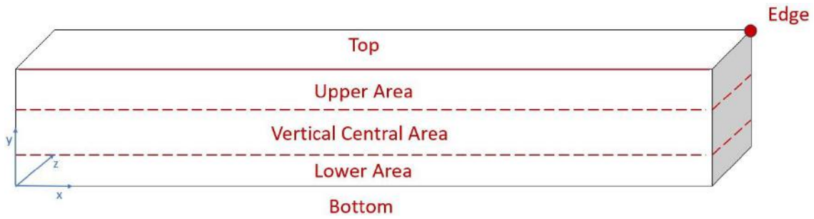
Figure 6: AOI types for representation of areas related to a components local x- and z-axis
