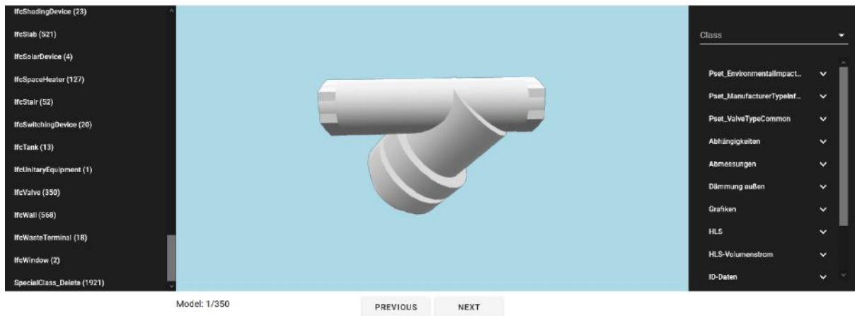
Figure 2: View of the tool used during the labelling process. The menu on the left allows switching between IFC classes. The menu on the right displays the current object's properties. The central canvas shows objects of the selected class in 3D.
