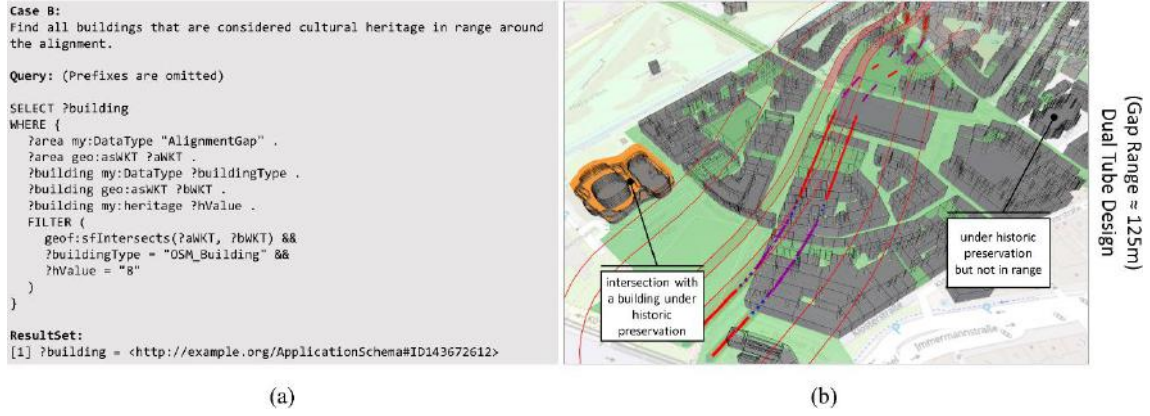
Figure 7: The query performed in Case B (a) and the results visualized in the project environment (b)
