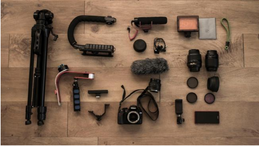
Fig. 13. Assembled over time, a DSLR kit's cost can be staggered. This setup was assembled over two years, and cost approximately $800. The camera is a Nikon D5500. It has 18–55mm, 55–200mm, and 50mm lenses alongside a range of filters, a lens hood, and wide-angle and macro adaptors. A gimbal allows for smooth handheld footage, as does a C-grip. A smartphone with a compatible lavalier microphone helps to round out this kit. Pictured, from left to right, top to bottom: tripod, c-grip, directional microphone, LED light panel, LED filters, focus pull, lens, lavalier microphone, a pair of lenses, cold shoes, Nikon D5500, lens, mobile phone grip, assorted lens filters, mobile phone.
