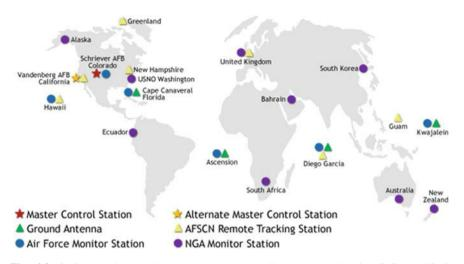
Fig. 4.3 GPS ground control segment (*source* http://www.gps.gov/multimedia/images/GPS-control-segment-map.pdf)
