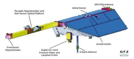
Fig. 3.3 CHAMP satellite structure (GFZ 2018)
