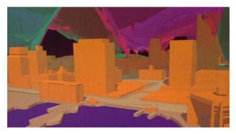
Fig. 16.4 Sunlight control modeling for Auckland city (1988), with the operative envelopes visualized as "stained glass" windows (Cadabra)
