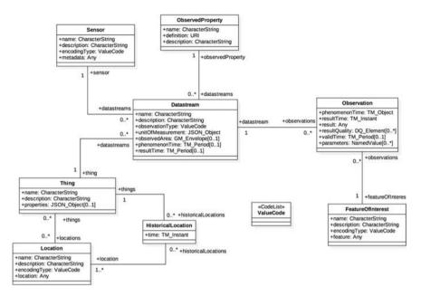
**Fig. 11.5** The SensorThings API data model. Each thing has a location (or some historical locations) in space and time. A collection of observations grouped by the same observed property and sensor is called a datastream. An observation is an event performed by a sensor that produces a value of an observed property of the feature of interest. *Source* OGC SensorThings API (http://docs. opengeospatial.org/is/15-078r6/15-078r6.html)
