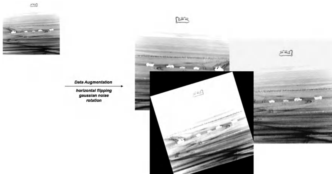
Figure 7. The data augmentation for each image, including horizontal flipping, Gaussian noise, rotation.
