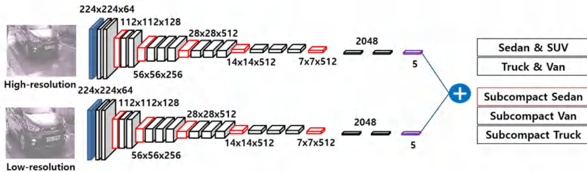
Figure 7. The architecture of the proposed multi-resolution network. Blue, black, and red cubes represent the resized input, convolution, and max-pool layers, respectively. Black and purple boxes are fully-connected and softmax layers, respectively.
