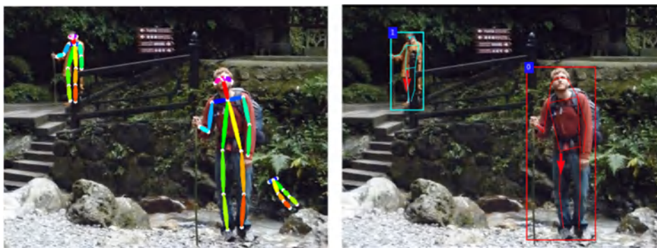
Figure 17. Examples of human pose estimation results generated by OpenPose [29] (left) and the proposed model (right).
