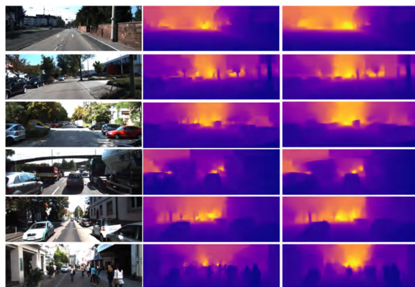
Figure A2. Example outcomes for the proposed method on KITTI. Columns from left to right: original RGB images, ground truth depth maps, and proposed model predicted depth maps. Colors indicate depth; yellow is far, and purple is close. Ground truth maps were interpolated from sparse measurements for better visualization.
